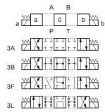
Code 5: 1 solenoid side A 2 positions (central + external) spring centering
