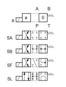
Code 1: 1 solenoid side A - 2 external positions with return spring
