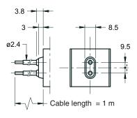
connection for DEUTSCH DT04-2P male connector type code K7
