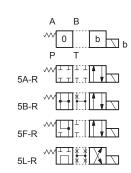
Code 1 Reverse Operator: 1 solenoid side B - 2 external positions with return spring
